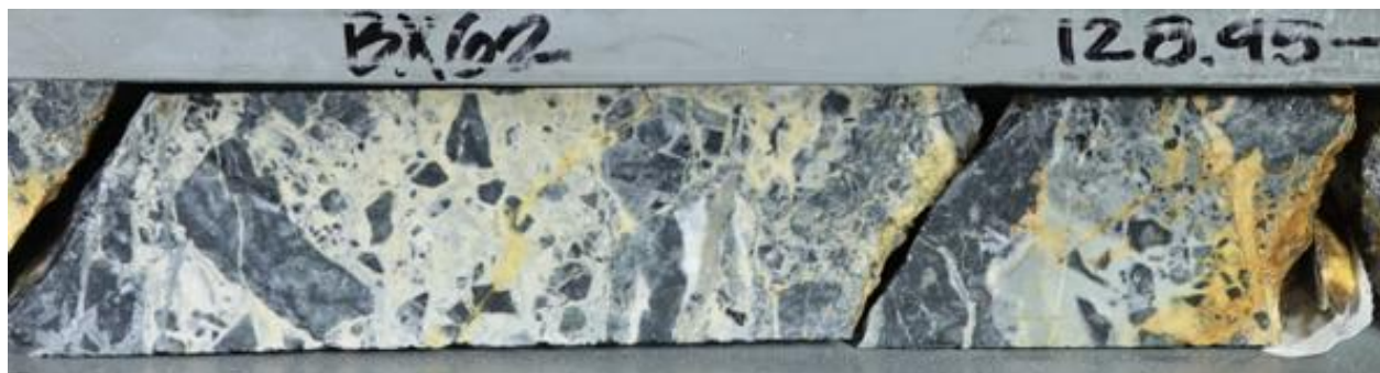
Figure 9: CMD26-054 angular wallrock clasts with silica cement at 128.45 m depth.
