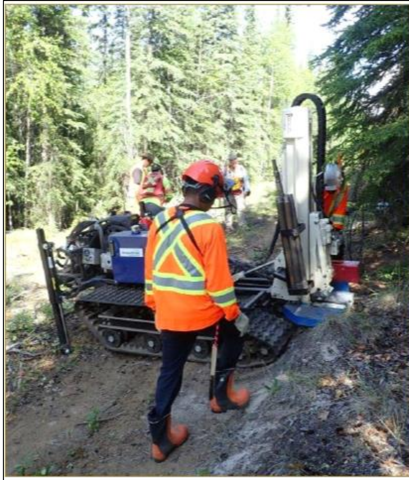
Figure 53: Geoprobe in operation (Tectonic Metals Inc. after Ground Truth Exploration Inc.)
